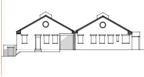
FRONT ELEVATION AS EXISTING Scale 1:100 @ A1
